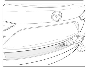
After all parts of kit are installed (rear bumper). Dry kit pieces using a heatgun.
