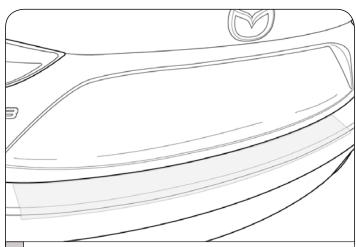
Repeat squeegee passes on the reverse side and go over a couple of times, Inspecting for excess water.
