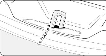
Locate the center of rear bumper piece and lift to spray alcohol in the center.
