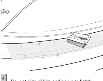
Re-wet side of film and begin to lightly stretch film into place. Hold in position with one hand and squeegee outward from the clean center in the direction pictured above.
